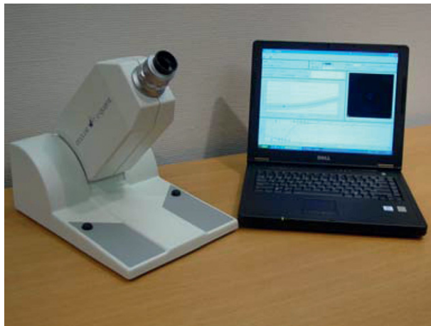
Figure 4 The C-Quant instrument from Oculus for measuring the amount of straylight in patient eyes.
